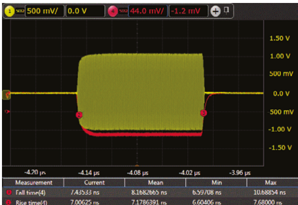
Pulse modulated signal and respective detector output signal. Maximum fall and build-up times are 7.5 ns.
